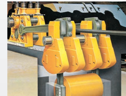
Cold pilger machine for rolling seamless tubes with special spherical roller bearings
