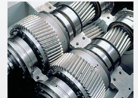
Rolling mill gearbox with tapered roller bearings and cylindrical roller bearings
