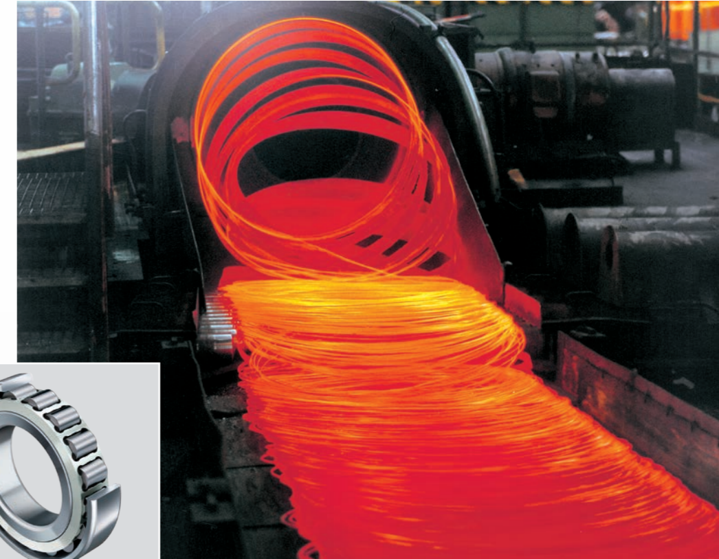
Wire rod block and laying head with special cylindrical roller bearings, angular contact ball bearings, and spindle bearings
