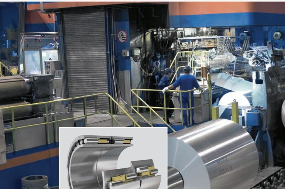
Multi-row cylindrical roller bearings in cold rolling stands
